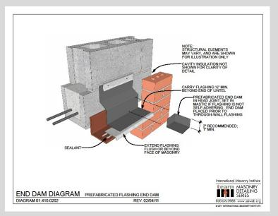
End dams are prefabricated or can be field-formed in the field with the flashing being used.
